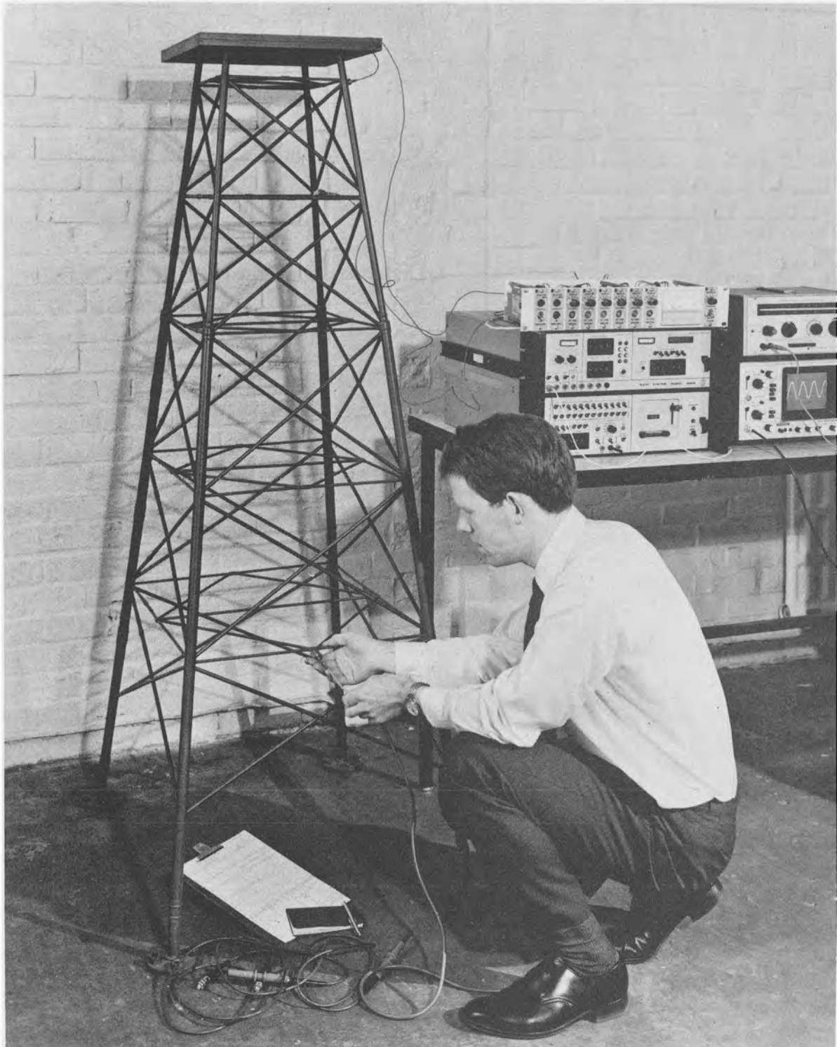
Fig.4. Model of a steel offshore platform under test to study vibration modes
