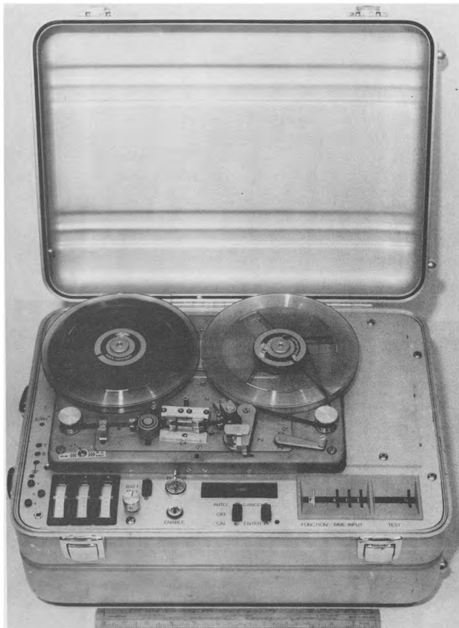
Fig.2. A portable seismic recorder designed for operation in remote areas. This equipment is commercially available
